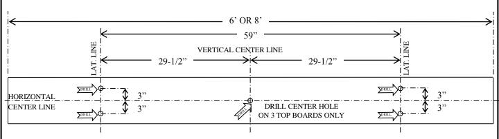
1.-Make sure all 5 boards are of consistent length, roughly 6' or 8' (two 6' and three 8' for ADA models).
